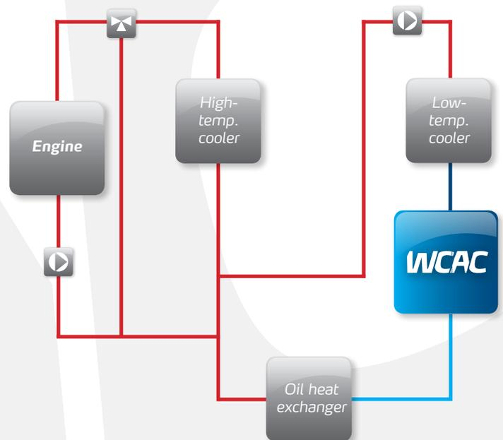
In addition, the WCAC system from Nissens is designed to comply with the applicable emission standards (Euro 6/Tier 4F), since a constant, lower charge air temperature leads to **lower emission levels**. This offers a vital contribution to ensuring environmental benefits and an increasing green focus in the market.
