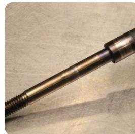
The surface of the turbo shaft is black and carbonized. Insufficient oil supply have caused overheating, thus making the steel color change. The blueish-to-yellowish color temperature is a heat tint caused by the overheating of the steel shaft.
