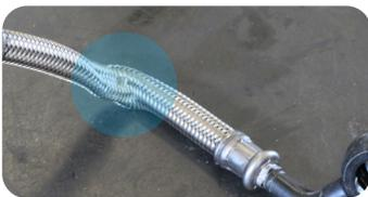
**Pipe Deformation > Oil supply disturbance:** Oil feedline deformation caused by careless installation. The line is tight but the deformation caused oil leakage, thus shortages in lubricant supply to the turbo.
