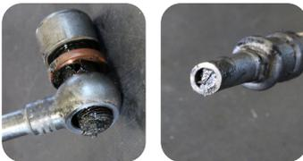
**Severe oil contamination > flow disturbance:** Severe oil contamination (sludge/carbonizing) caused oil feed line restrictions - visible on the banjo fitting, as the severe contamination built up inside of the pipe.
