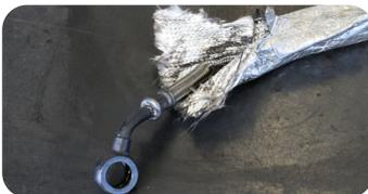
**Lack of heat protection > flow disturbance:** torn, deteriorated heat protection shield of the OFF may lead to inner flow restriction due to oil carbonizing and cause severe contamination to build up inside of the pipe.
