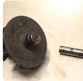
Broken shaft caused by a lack of lubrication. The high rotation speed and frictions within the moving parts have caused the temperature to increase extremely, the shaft to warm up, and ultimately break by seizing.
