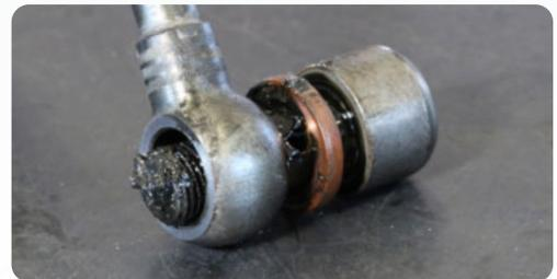
**Oil supply disturbance:** Severe oil contamination (sludge/ carbonizing) caused oil feed line restrictions visible on banjo fitting.
