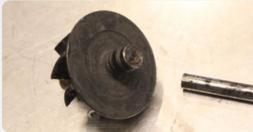
**Insufficient lubrication:** Broken shaft caused by lack of lubrication. The high rotation speed and frictions within the moving parts have caused the temperature to increase extremely, the shaft to warm up, and ultimately break by seizing.
