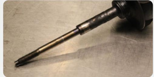
**Insufficient lubrication:** The surface of the turbo shaft is black and carbonized. Insufficient oil supply have caused overheating at first, thus making the steel color change. The blueish-to-yellowish color temperature is a heat tint caused by overheating of the shaft steel. Next, the remaining oil will start coking on the surface, making the black sinters.
