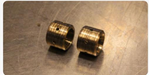
**Oil contamination:** The clearly visible grooves on the journal bearing surface arise from frictions and excessive material abrasion provoked by impurities in the oil. Despite the presence of oil, shaft of this turbo get seized.
