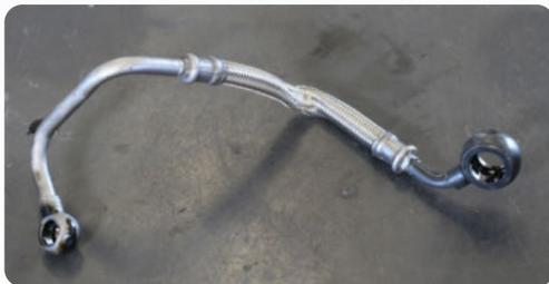
**Oil supply disturbance:** Oil feedline deformation caused by careless installation. The line is tight but the deformation caused oil thus shortages in lubricant supply to the turbo.
